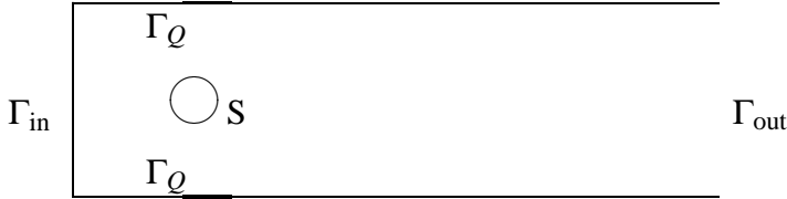
Figure 5. Configuration of the drag minimization problem
